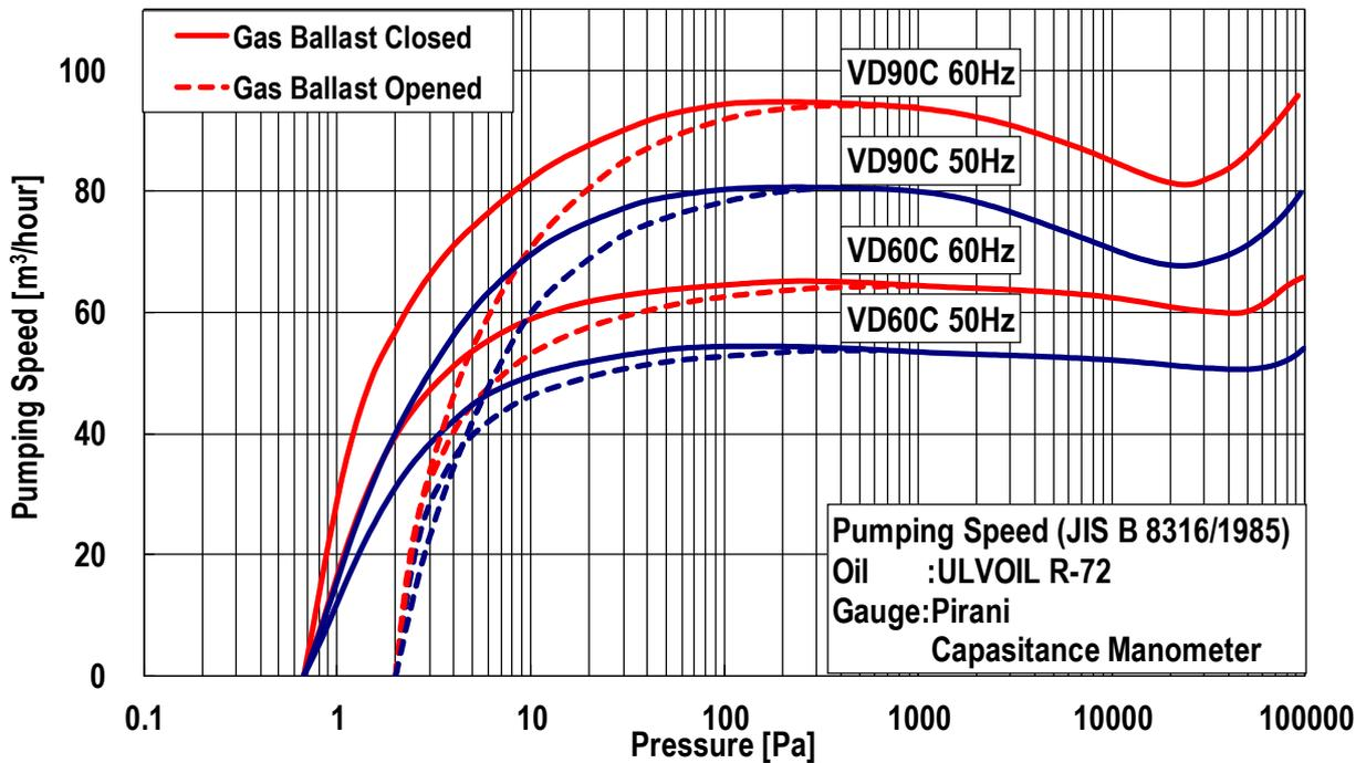
Fig. 13 Pumping speed curves - MODEL VD60C/VD90C
