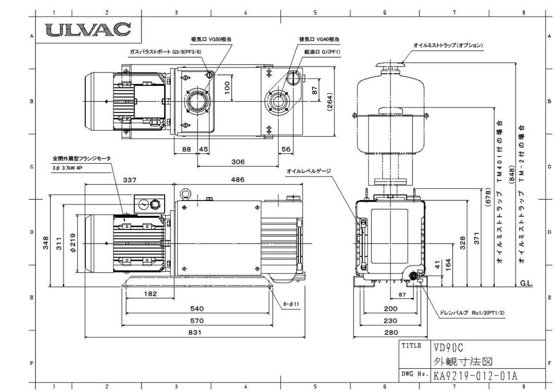
Fig. 7 Dimensional drawing VD90C
