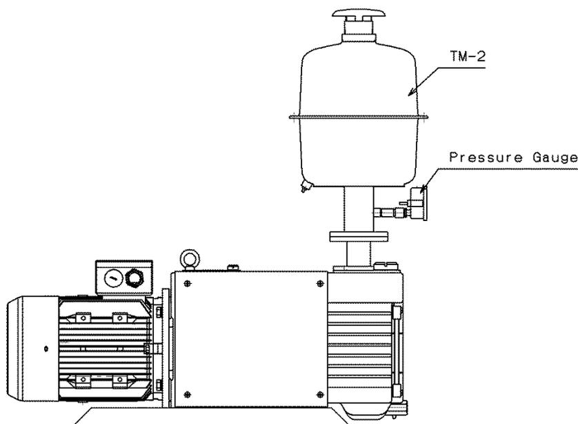
Fig. 18 Installation example VD90C
