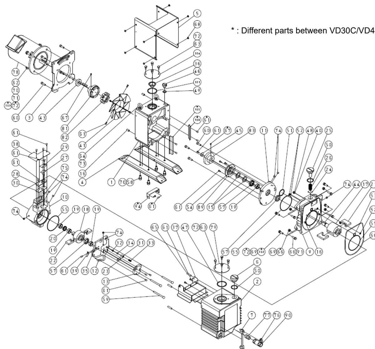
Fig. 20 Exploded perspective view
