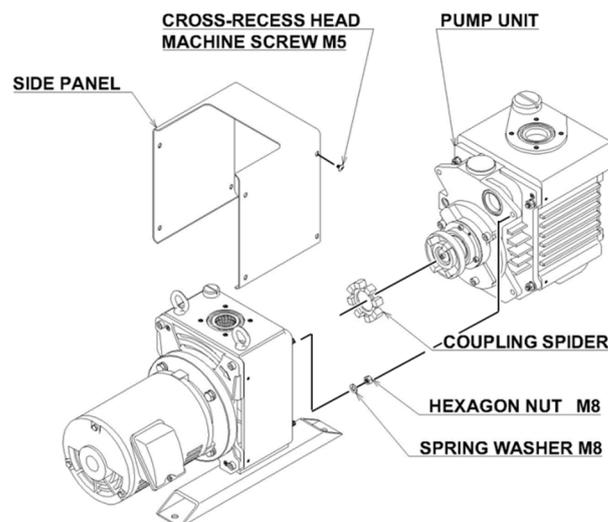
Fig. 19 Replacement of coupling spider
