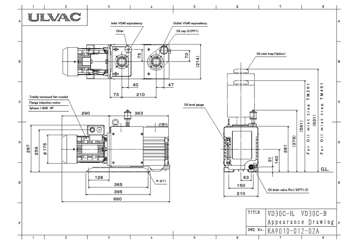
Fig. 8 Dimensional drawing VD30C-H, VD30C-B
