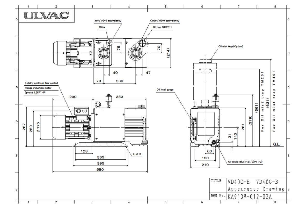
Fig. 9 Dimensional drawing VD40C-H, VD40C-B
