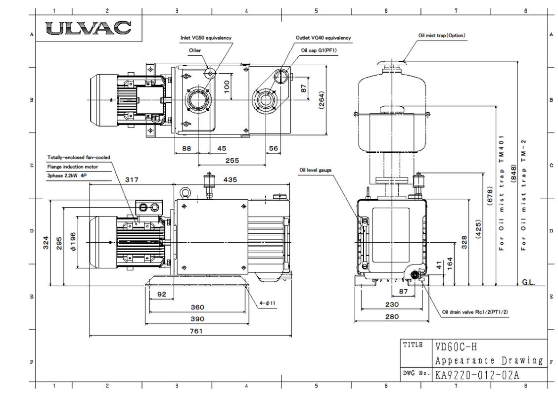
Fig. 10 Dimensional drawing VD60C-H
