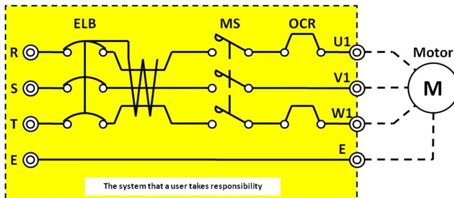
Fig. 16 Recommended connection diagram
