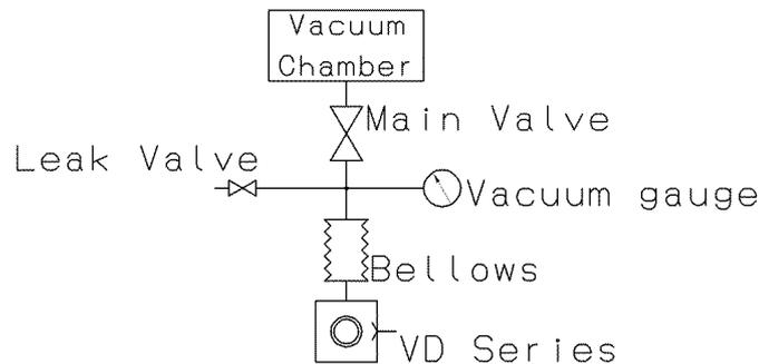
**Fig. 15 Connection to vacuum chamber (example)**
