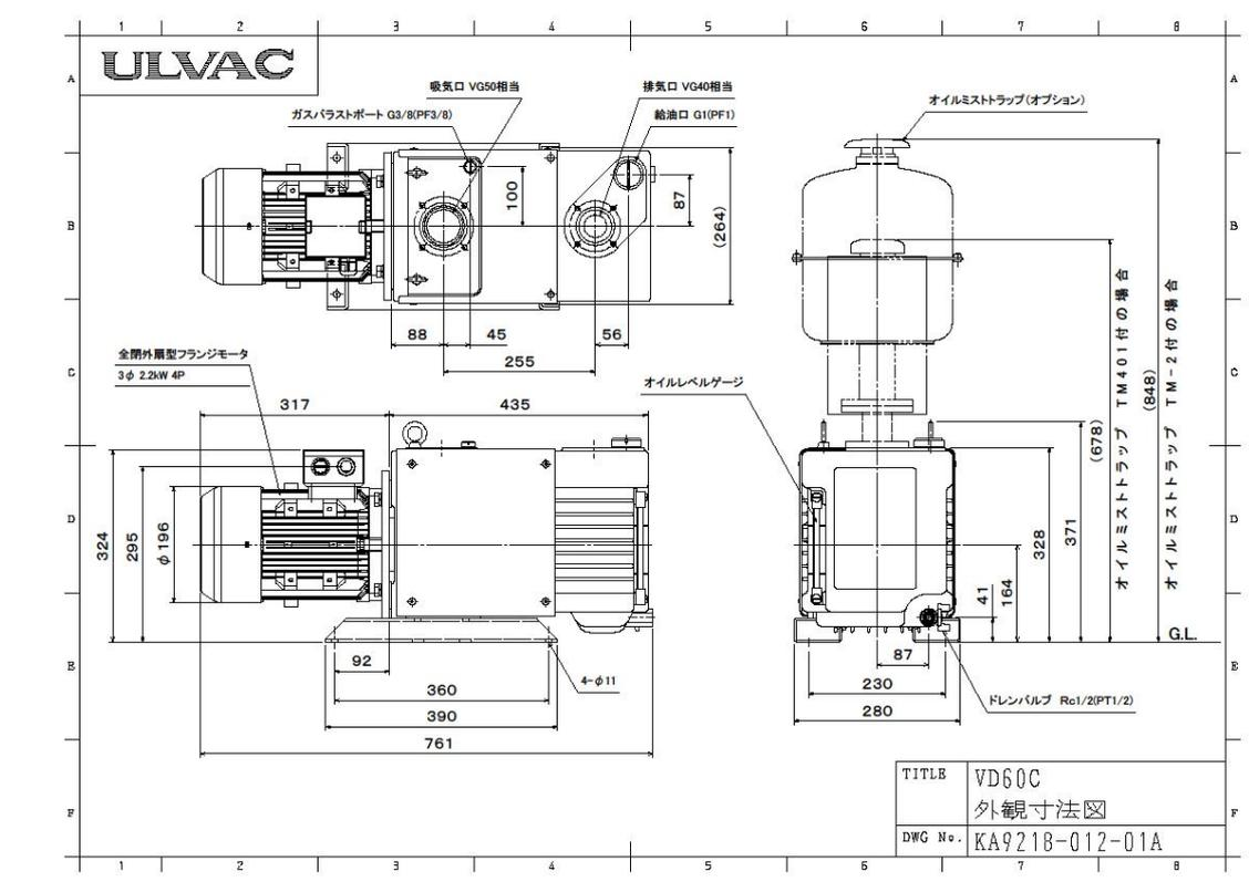
Fig. 6 Dimensional drawing VD60C
