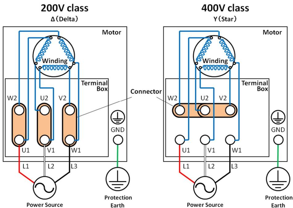
Fig. 17 Electrical wiring diagram
