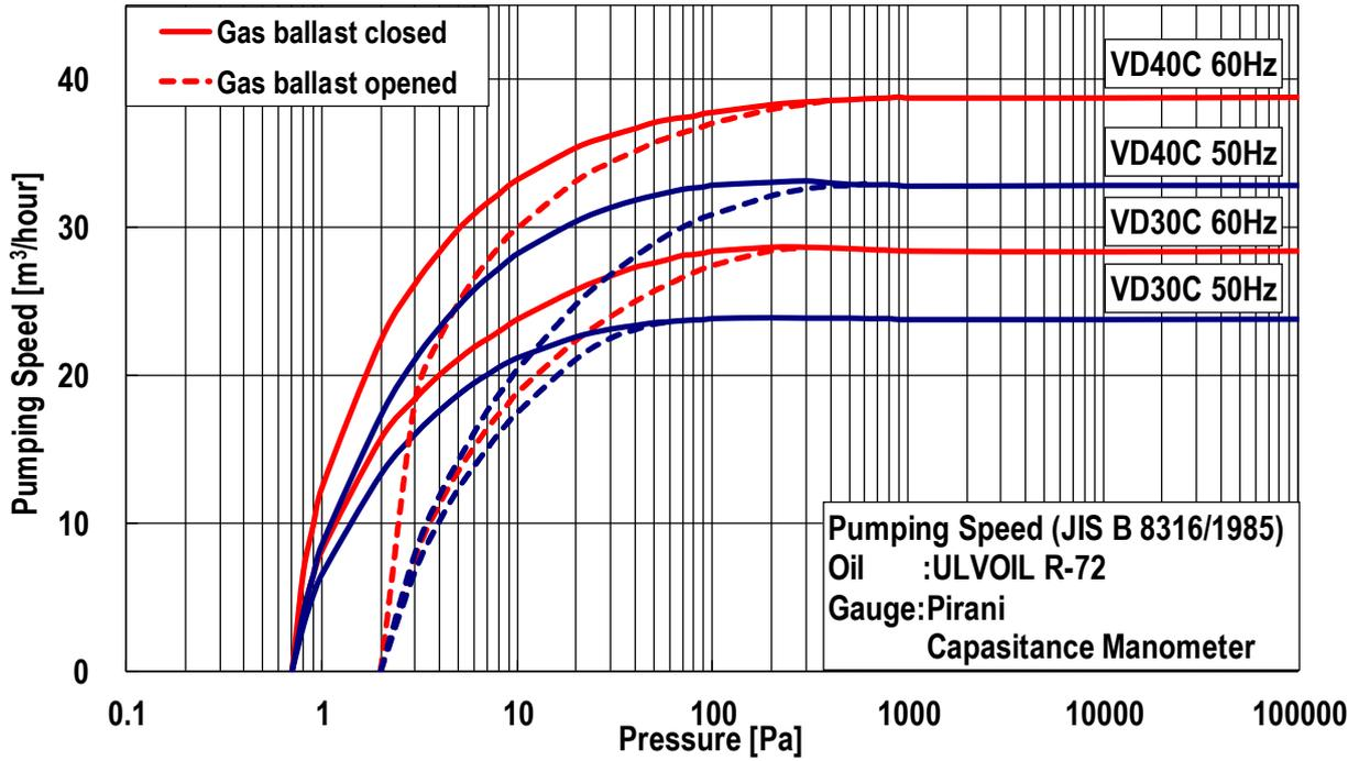
Fig. 12 Pumping speed curves - MODEL VD30C/VD40C
