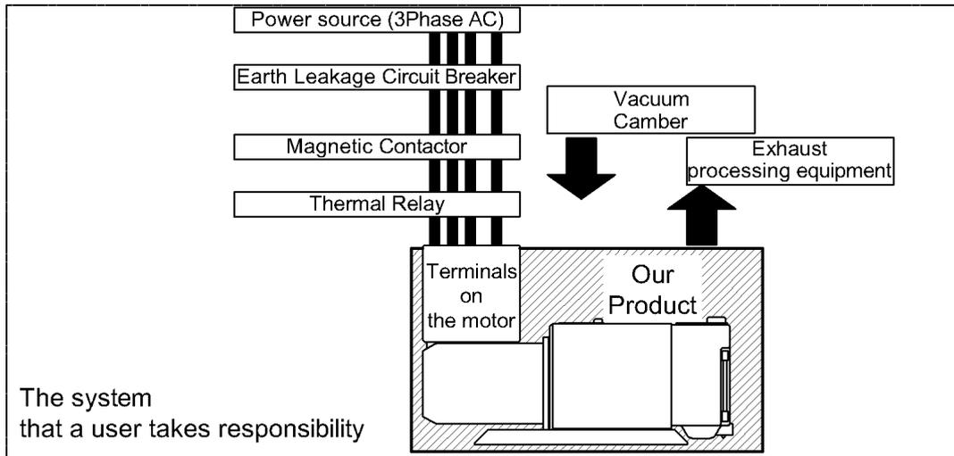
Fig. 3 Location of vacuum pump in host device
